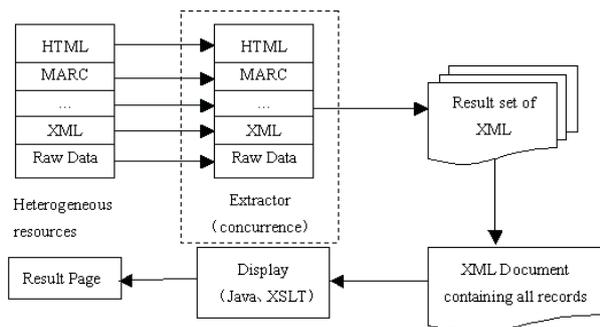
Fig. 2. Merging Module
