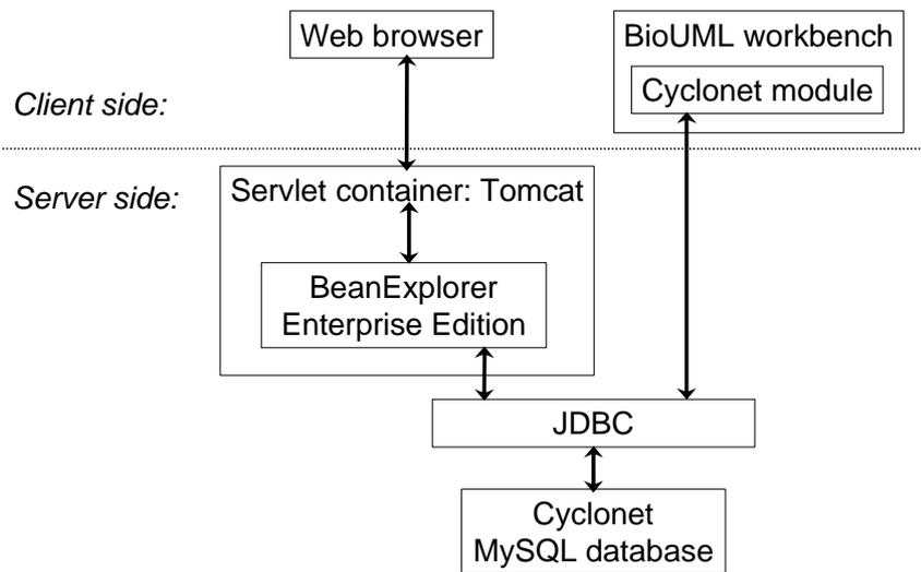
Figure 1. Cyclonet system architecture.
